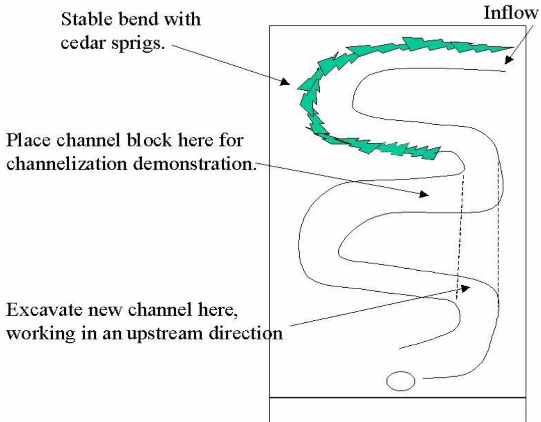
Figure 2. Placement of stable bend and channelization demonstration on the model stream.
