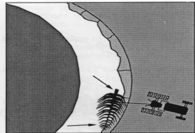
3. Tree is pulled tightly against bank and anchored at points shown by arrows.
